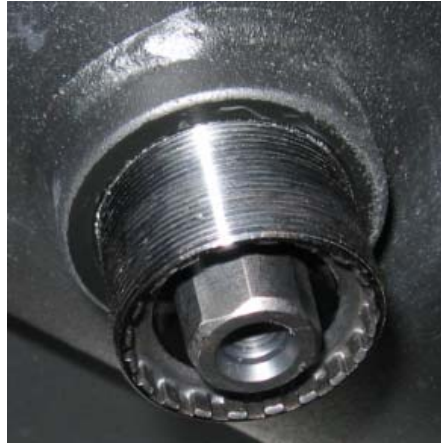
Install Left Side Cup 1-2 threads.
