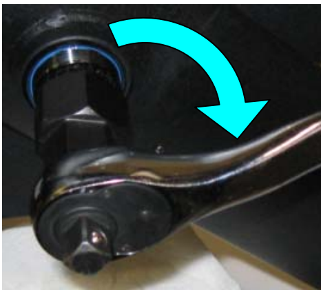
Thread in left cup completely. (clockwise) and torque to 175 in*lbs
