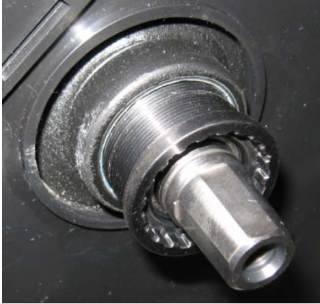
Install Right Side Cartridge 1-2 threads.
