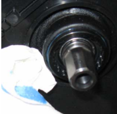
Wipe away excess Loctite.
