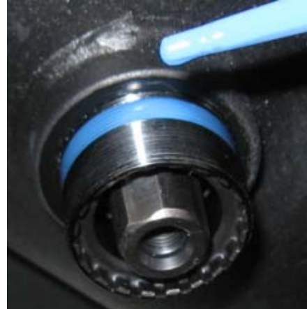
Apply Loctite 242 to Left Cup. * Again, apply closer to the frame so as you install the cup the Loctite will spread across all threads.
